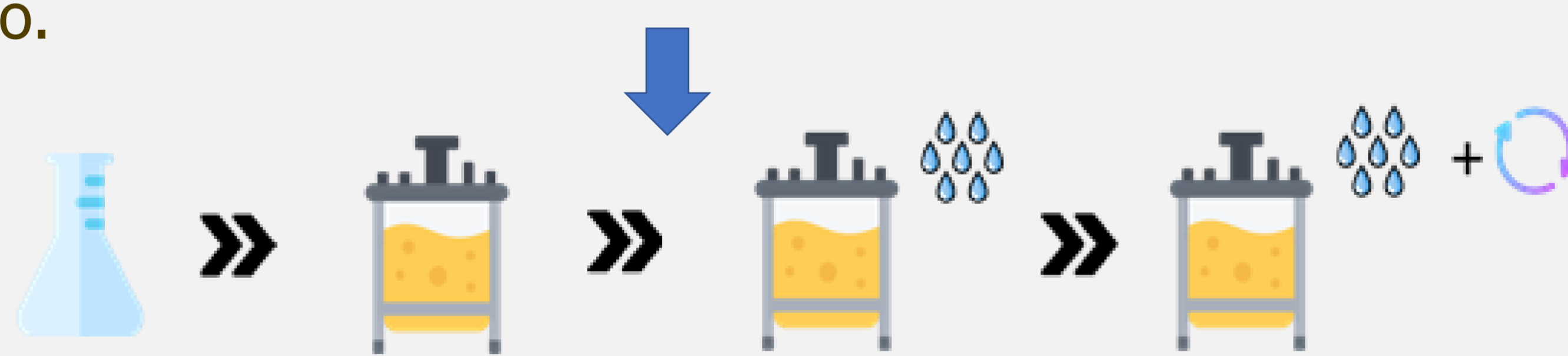
Figura 4: Preinoculum (8 h) → Batch (4 h) → Induced fed-batch (24 h) → Induced fed-batch + harvesting (40 h)
